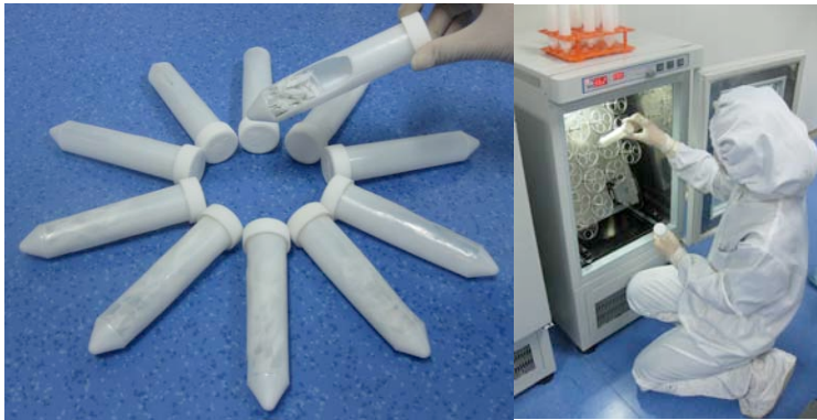
Figure 7. Single-use 20ml work volume mini-bioreactor vessels filled with 1.0 gram of polymer cell-anchorage carriers (left) and working mini-bioreactor for perfusion scale-up and media optimization (right).
